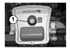
When the preheating pilot lamp has gone out, turn the ignition key to position 2 and start the engine. When the engine has started, the pilot lamps (1) must go out.
