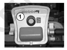
The driving speed as well as the direction of travel are controlled by means of the rocker switch (1).
