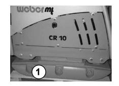
Remove both oil drain screws (1) and drain the oil. To refill, slightly tilt the machine and add fresh oil through the drain hole according to the fluid chart.
