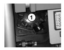
Screw the hose down to the drain valve of the hydraulic tank (1) and drain the oil.
